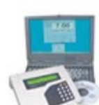
DAS for communication to computer
